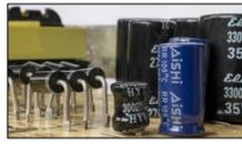
Know what a circuit board capacitor does? Technically, it's a passive, two-terminal, electrical component that stores energy in an electrostatic field, so when there's an electrical potential difference across the conductors of a circuit, a static electric field develops across the capacitor's dielectric, causing positive and negative charges to collect on separate plates.
